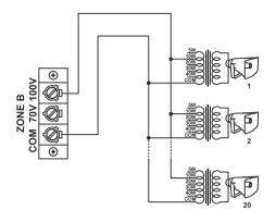
On Zone B, 20 SUH-40XT Horn Speakers with 100V LMT connected at 10W can be operated.
