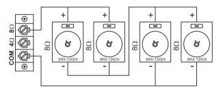
Resultant Impedance =  $(8 \text{ ohm/2}) \times 2 = 8 \text{ ohm}$
