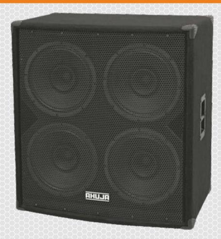
Sturdy & rugged carpet covered bass reflex cabinet built around 4 nos high quality 12" 200W dual cone speakers. Features high efficiency, high sound pressure level, & unmatched bass. Tuned for optimum performance, and having a high power handling capacity of 800 watts RMS, this is an ideal cabinet speaker for large gatherings and for use with high power amplifiers.
