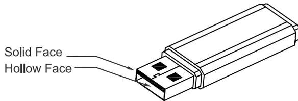
Any forceful insertion in wrong direction will damage the connector.
