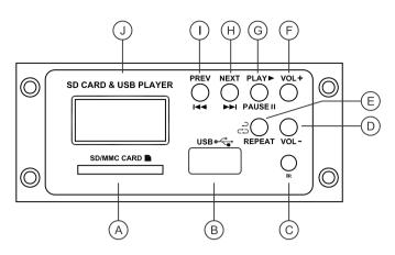
A. SD/MMC Card Connector: Insert the SD/MMC Card into its appropriate slot to play. When taking out the card, pull the card to take out.
